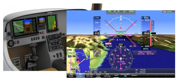
With ever denser air traffic, collision detection and avoidance capabilities are ever more relevant for the safety of general aviation. The lowest airspace band will be shared with more and UAS (Drones). See and avoid is no longer an option. Airplanes over 5700 kg will have a mandatory collision avoidance system based on Mode S transponders and ADS-B. Alternative systems like FLARM and 4G/5G mobile phone solutions are competing to enter the market for GA.
