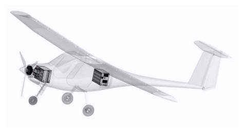
The holy grail for zero emission airplanes is the direct electric powertrain. Many developments are underway and the first airplane - the Velis-Electro from Slovenian company Pipistrel - is EASA certifed. Designs not conceivable before will come with multiple computer controlled engines and induce novel airplane.
